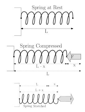
The relationship between the change x of the length of a spring from compression or stretching caused by a force F is
